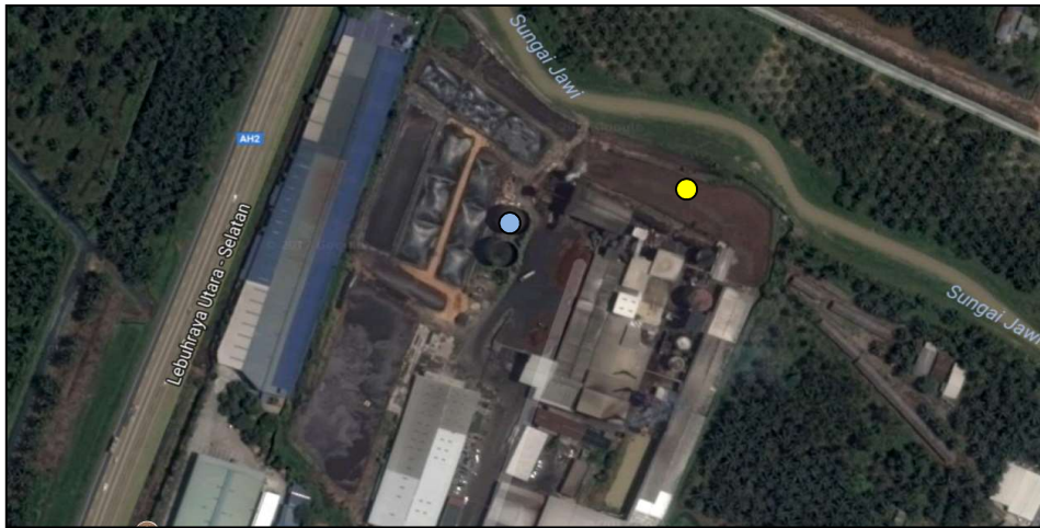
Fig. 2. The covered anaerobic lagoons at Mill B. On-site odour assessment was performed nearby the anaerobic ponds (●), while odour samples were collected from the cooling pond (●, with an estimated size of 161 m x 30 m = 4830 m 2 )
